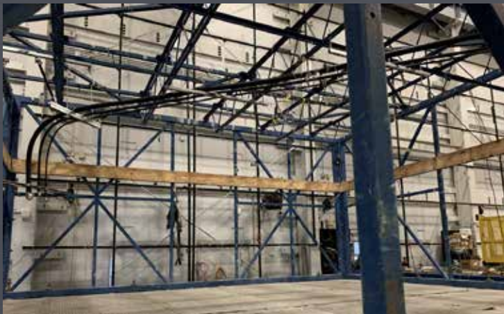
TracPipe System CSST in seismic test rig.
