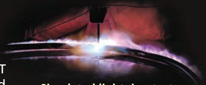
Simulated lightning test with no product failure
