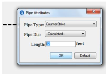
Select the pipe type, usually *CounterStrike*, and specify the length of the pipe in feet. The pipe type will be remembered for next time. Click *OK*. *Pipe Dia.* is for existing pipes in legacy systems or for forcing explicit sizes.
